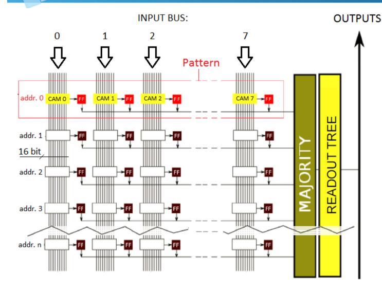
The **INPUT** buses could be **asynchronous**: the **matches** are **independent**!
