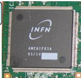
**Standard Cell 0.18  $\mu$ m**  $\rightarrow$  5000 pattern/AM chip
